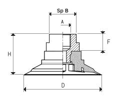
Note: The force of the vacuum cups indicated in the table represents 1/3 of the value of the theoretical force calculated at a level of vacuum of -75 KPa and a factor of safety 3. Transformation ratio: N (newton) = Kg x 9.81 (force of gravity) inch =  $\frac{mm}{25.4}$ ; pounds =  $\frac{g}{453.6}$  =  $\frac{Kg}{0.4536}$  Adapters for GAS - NPT threading available on page 1.130
